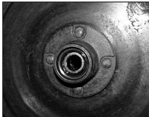
▲ Case IH Seal/bearing in John Deere drill after 3000 acres
