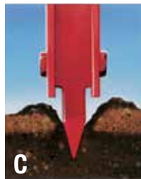
C Check furrow forming point depth ( C ).
